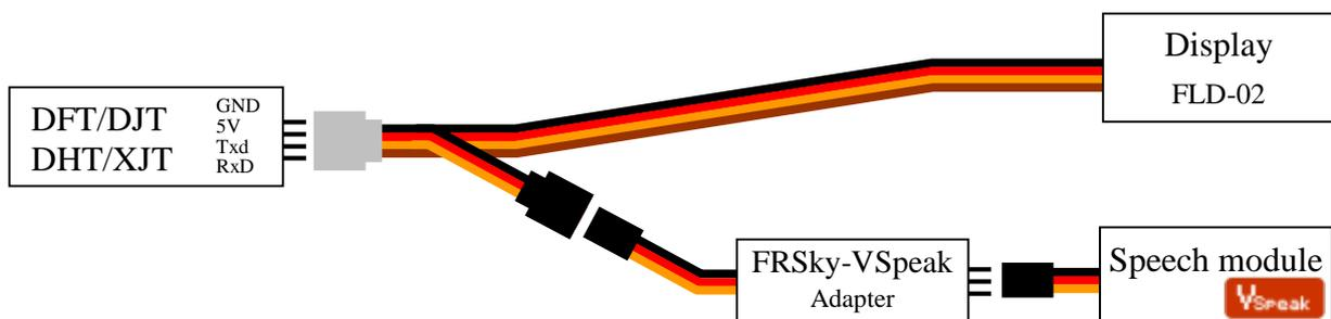
The operation with the display FLD-02 is always necessary when the parameters are set for the alarms of the analog values 1 and 2 and the Rx and Tx signals (see section 3.2.1).
